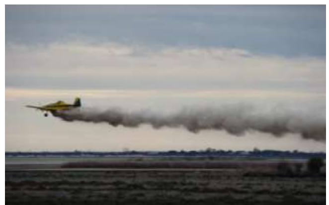
Aerial Limestone dosing
